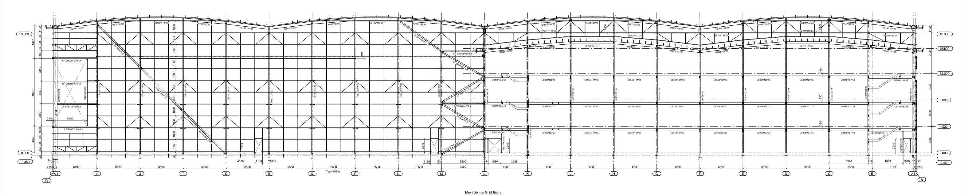
Rail SPEC Metsec Sleeved system OUS Rails 202C15 DTW = Diagonal tie wire SRS = Side rail support TS = Tubular Strut Cleader angle 100x100 supplied by Caunton
