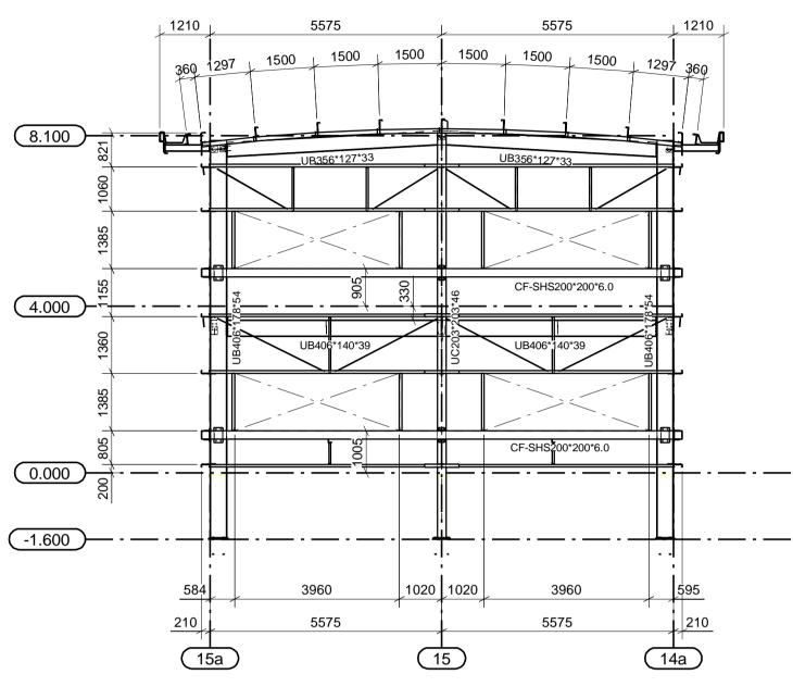
Elevation on Grid line Y
