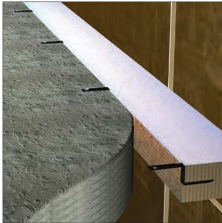
FJ220 with Z-clips on a non-combustible curtain wall
