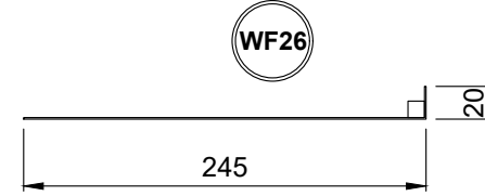
0.7mm THK CILL FLASHING COLOUR: HPS200 - ANTHRACITE
